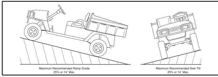
Fig. 2 Vehicle Incline Specifications
